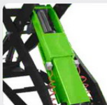
With hydraulic lock and mechanical dual-gear safety-claw lock double safety device, automatically open when lowering. By lock operation can has the safety-claw located adversely, safe & reliable.
