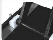
Sliding blocks adopt oil free super-wearable materials.
